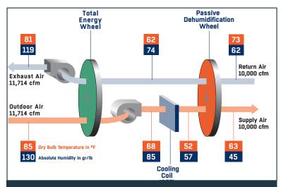
Operating at peak space latent load providing 70.1 tons of total cooling at a sensible heat ratio (SHR) of 0.27 using only 33.8 tons of refrigeration input. The dew point delivered to the space is 45.4°F. A conventional system with the same leaving coil temperature will NOT deliver the samedew point. It would require 81.1 tons of refrigeration and 156 MBtuh to achieve the same leaving coil condition.
