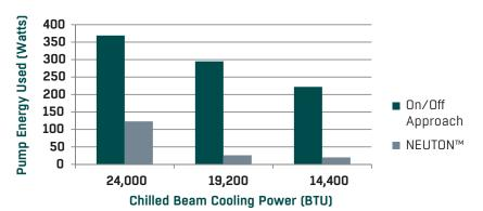
Standard efficiency pump (on/off) vs high efficiency ECM variable speed pump served by the NEUTON™ pump module control logic
