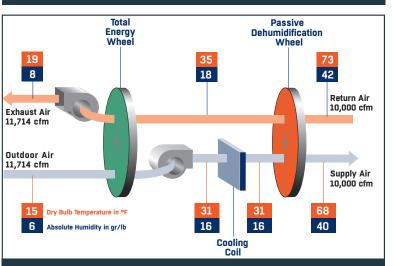
Operating in heating mode providing 573 MBtuh of energy and 219 MBtuh of humidification.
