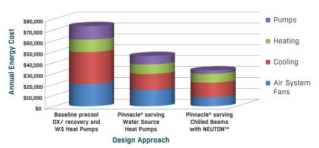
Energy modeling completed for a high school project comparing three design approaches which highlights the energy savings offered by the 3fficiency™ system, even over the efficient Pinnacle I<sup>®</sup> serving water source heat pumps.
