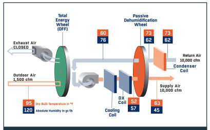
Operating in unoccupied mode. The system can operate in 100% recirculation mode and with very little refrigeration input effectively controlling the indoor humidity, to comply with ASHRAE 62.1 addendum ae.
