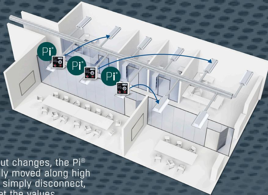
When the office layout changes, the Pi<sup>®</sup> actuator can be easily moved along high occupancy rooms — simply disconnect, re-connect and re-set the values.
