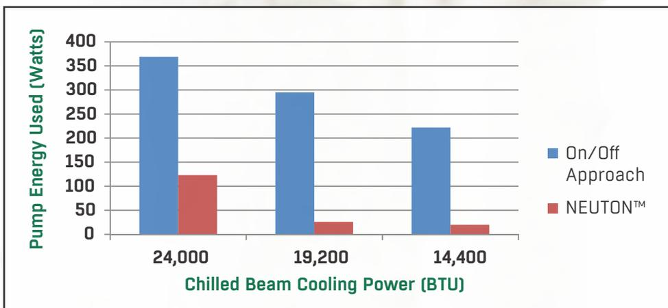
**Standard efficiency pump (on/off) vs. high efficiency ECM variable speed pump served by NEUTON control logic**
