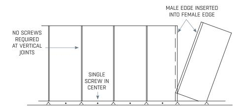
FLÄKTGROUP<sup>®</sup> SEMCO<sup>®</sup>'S FIRE RATED PANELS INCORPORATE A PROVEN TONGUE-AND-GROVE JOINT, DESIGNED TO REDUCE INSTALLATION TIME AND REDUCE COSTS.
